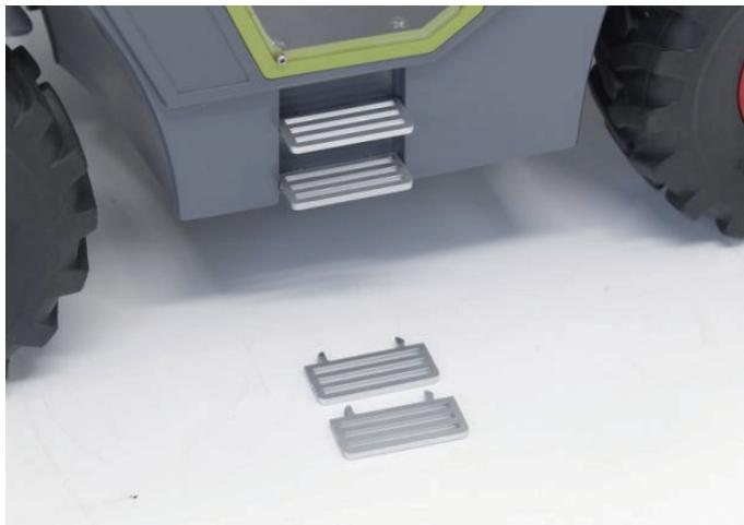
1. Cab pedal installation: pay attention to the front and back (the chamfered side is the upper side), and you can just click it in directly.
