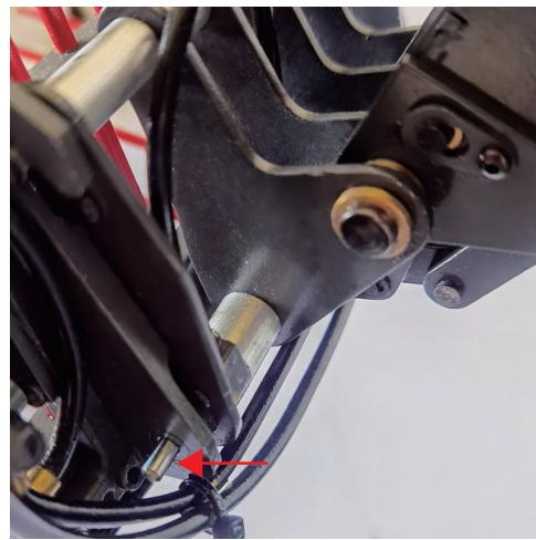
3. Put the hydraulic claw on the hook first, press down to the position, open the remote control oil pump channel CH5, and then open the remote control CH10, confirm that the pin at the lower end of the claw is in place.
