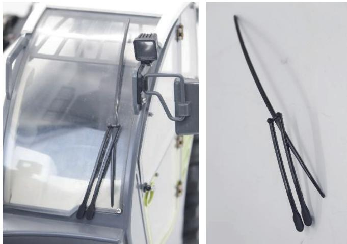
2. Wiper installation: directly press it to the hole in the cab, or use glue to stick it.
