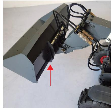
5. Install the bucket, hang the hook on the bucket on the shelf, open the oil pump channel CH5, open the channel CH10, and insert the fixing pin into the fixing hole of the bucket to complete the installation (it is best to move the male end of the quick release cylinder to the top to make the bevel angles of the left and right pipes the same).
