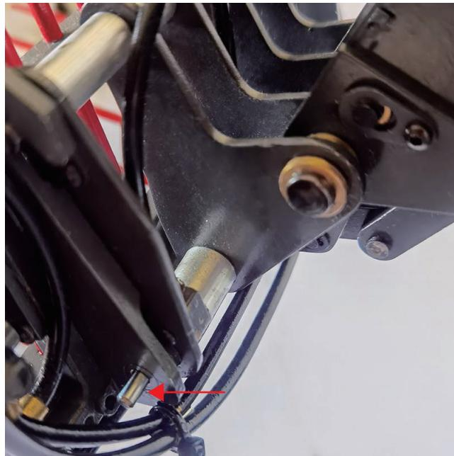
1. Turn on the remote control CH10, shrink the pin.
