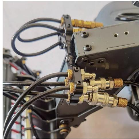
3. Close the oil pump channel CH5, pull out the quick release joint connected with the claw backwards, and separate.
