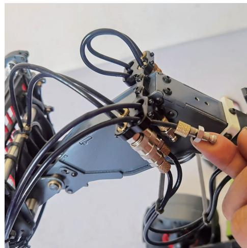
4. Loosen the fixed machine screw and take out the hydraulic quick-change male end of the claw (It is better to move the male end of the quick-release cylinder to the top so that the angles of the left and right pipes are the same).
