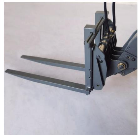
6. Install the fork in the same way as the bucket (it is better to move the male end of the quick-release cylinder to the top so that the corners of the left and right pipes are the same).
