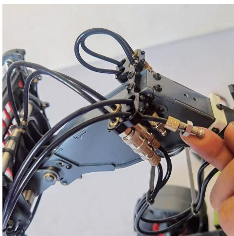
1. Take out the claws, confirm that the oil pipe is tightly connected with the oil nipple and hydraulic quick-change male connector, and pass the oil pipe through the oil pipe bracket.
