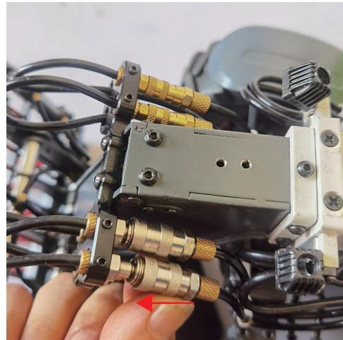
2. Tighten the hydraulic quick-change male head (by tighten the two M3 screws above), confirm the sequence of the oil circuit (action sequence), and push the hydraulic quick-change female head into the male head.
