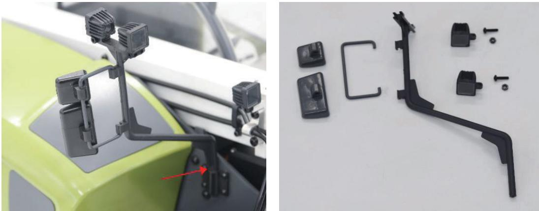
4. Rear frame installation: pay attention to the fit of the installation slot and the bracket rod.
