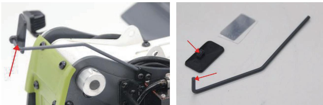
7. Auxiliary mirror installation: the bracket rod is linked to the frame hole, and then fixed to the bracket.
